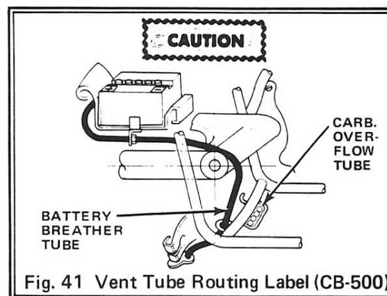
Fig. 41 Vent Tube Routing Label (CB-500)
