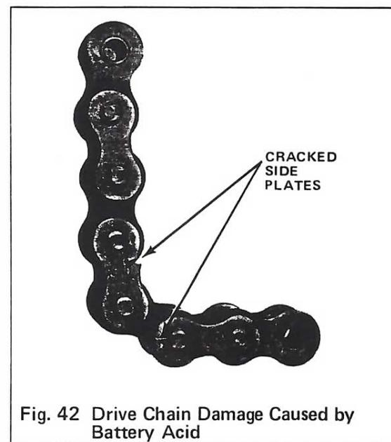
Fig. 42 Drive Chain Damage Caused by Battery Acid
