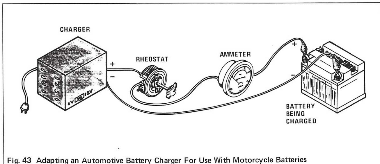
Fig. 43 Adapting an Automotive Battery Charger For Use With Motorcycle Batteries
