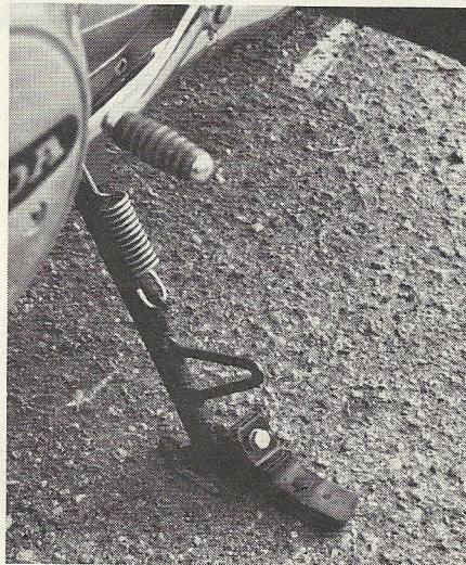
The rubber tab added to the side stand is designed to drag and fold the stand up if you leave it down accidentally. It only worked about half the time.
