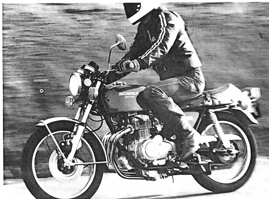
The axle carrier on the swing arm isn't a separate piece; it's stamped from the arm itself.
